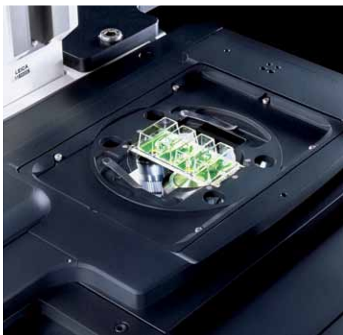
SuperZ Galvo focus for ultra-fast and highly precise z-stacking.
