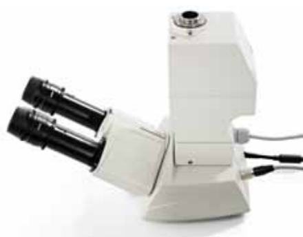
Fig. 20 Trinocular Tube DM FS with 3-position magnification changer
