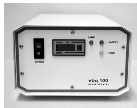
Fig. 67 Supply unit Hg 100 W
