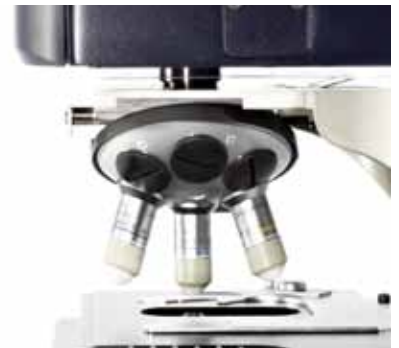
Fig. 19 Motorized objective nosepiece for up to 6 objectives
