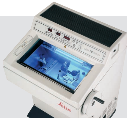
The Leica CM1900 UV rapid sectioning cryostat: Extremely rapid freezing through a quick freezing shelf for up to ten specimens and independent specimen cooling for brief and frequent temperature changes.
