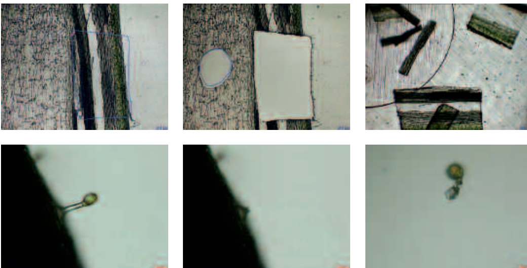
Fig. 8–10 (from left to right): Laser Microdissection of long, large areas in the range of mm 2 in a single piece from Arabidopsis stem-section (60 µm thick): – before microdissection – after microdissection – inspection mode
