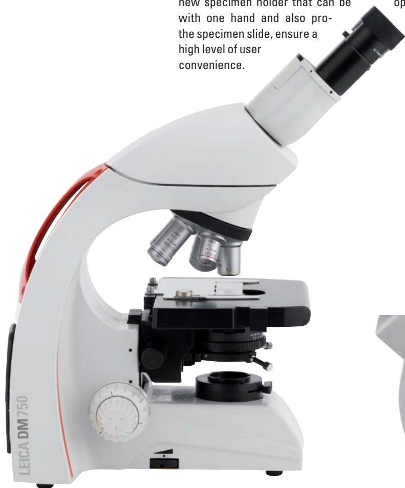
Fig. 1: Equipped with high-quality optic components, the Leica DM750 has wide application potential.
