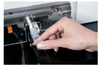
Fig. 2 and 3: The Leica EM PACT2 + RTS high-pressure freezer, suitable for standard high pressure freezing and CLEM experiments. Its operation is very easy: All you need to do is insert the rapid loader, the machine will do the rest.
