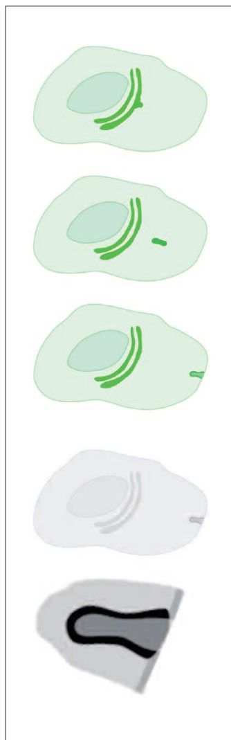
Fig. 1: Schematic model of a CLEM experiment. In a modern CLEM experiment a sample is first studied live under the light microscope (Green cells). A structure inside the cells can be followed (arrows). When an interesting event occurs the sample is fixed and processed for electron microscopy. The same cell is traced back in the EM (grey image) and the structure and event of interest can be studied at high resolution.
