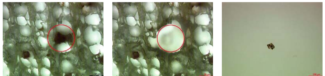
Fig. 1–3 (from left to right): Laser Microdissection of small area of spruce section (73 µm thick): – before microdissection – after microdissection – inspection mode
