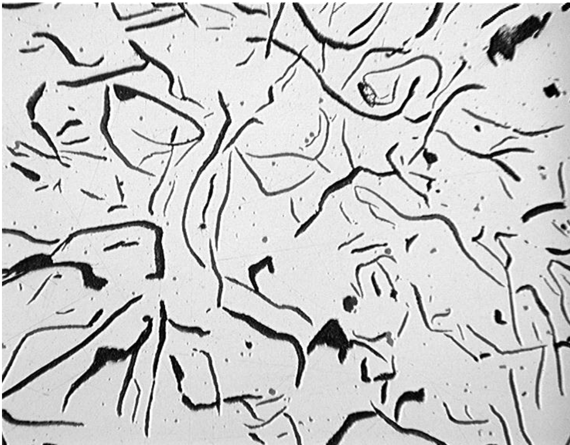
Figure 4 An image of graphite nodules flake graphite.
