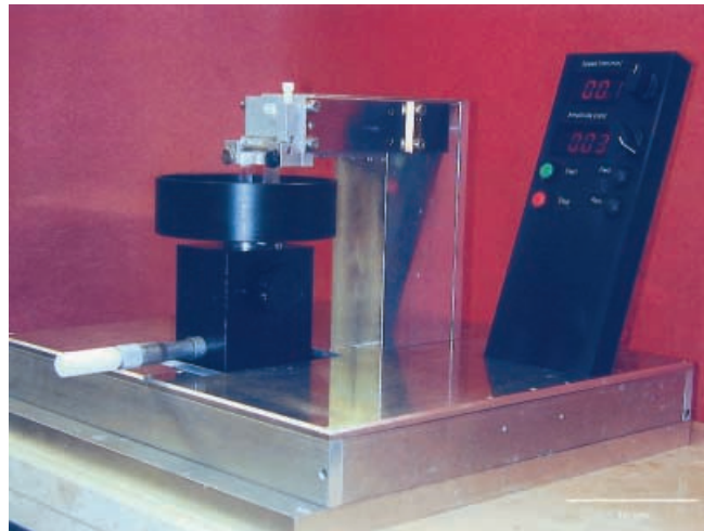
Fig. 3 Photograph of the vibroslicer. A probe holder mounted on a height-adjustable block is visible in the centre . Height adjustment of the probe holder is made manually by means of the micrometer screw on the front ( left in the figure). DC motor, tachogenerator and gear used for generating horizontal movement of the sample holder are situated within the main body, below the folded cover . The oblique panel on the right contains control and display elements. The block of stone (mass \approx 40 kg) on which the vibroslicer is mounted is visible below the slicer
