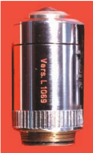
Fig. 9: Leitz (Leica) early (1967) prototype ("Versuchs") oil immersion objective x40 with a NA 1.30 developed for trial experiments in fluorescence epi-illumination technology.
