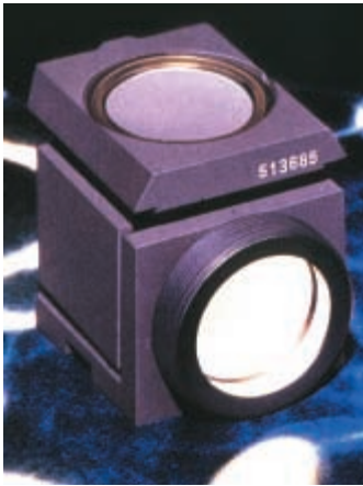
Fig. 4: Complete Leitz (Leica) filter cube (block) for fluorescence microscopy containing: excitation filter, dichroic beam splitter and emission (barrier) filter.
