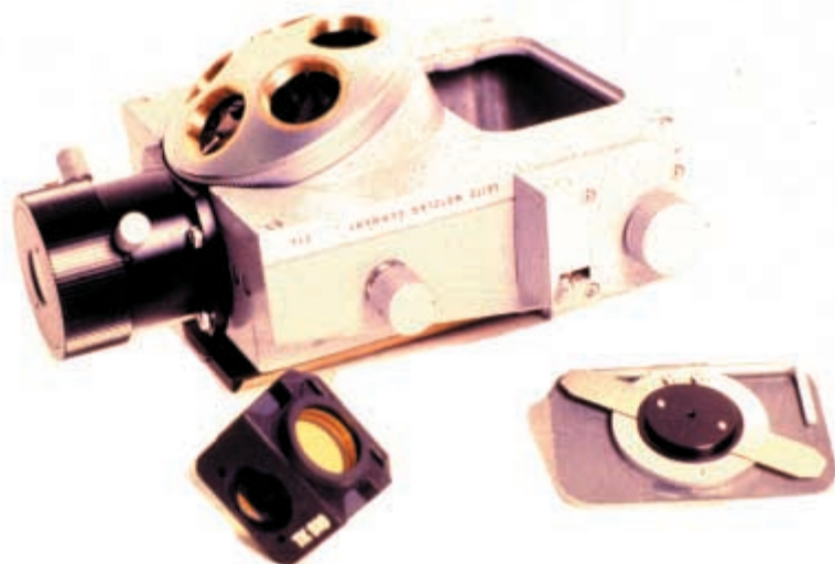
Fig. 1c: Leitz epi-illuminator with four exchangeable filter cubes (blocks) [Kraft, 1972].
