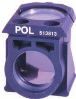
Fig. 12: A filter cube (block) for reflection contrast microscopy, containing a polarizer, a neutral (50 %) beam-splitter and an analyzer. This filter cube (block) can be inserted into one of the positions of a Leica epi-illuminator for fluorescence microscopy.
