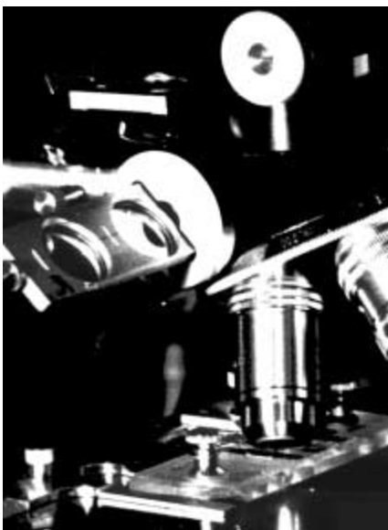
Fig. 1b: Leitz prototype (not commercialized) multi-wavelength epi-illuminator with four dichroic beam-splitters mounted in a slider (Ploem, 1967).
