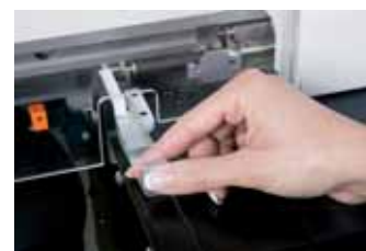
Fig. 2 and 3: The Leica EM PACT2 + RTS high-pressure freezer, suitable for standard high pressure freezing and CLEM experiments. Its operation is very easy: All you need to do is insert the rapid loader, the machine will do the rest.
