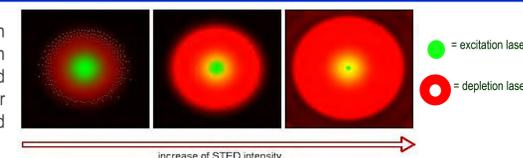
**Figure 6:** The excitation beam and STED depletion beam
