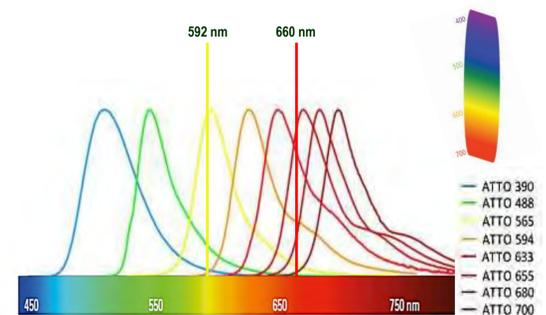
**Figure 7:** Dye spectra examples from ATTO with the Leica STED lasers at 592 nm and 660 nm
