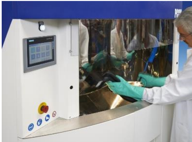
Pressure rinsing method applied to a reservoir and a collector
