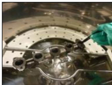
Pressure rinsing method applied to a reservoir and a collector
