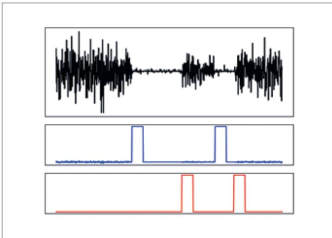
Precisely synchronize your functional imaging to external stimuli. External sensor data (black) used to control imaging by sending stimuli triggers (red) and receiving imaging triggers (blue).
