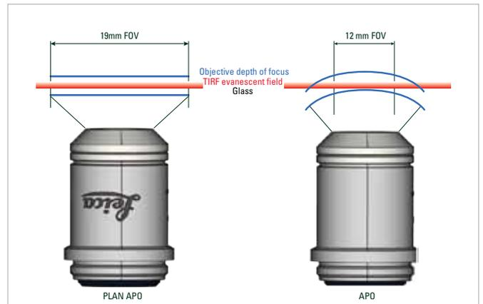
Dedicated TIRF objectives – Leica’s high quality PLAN APO corrected TIRF objectives enable a homogenous TIRF imaging over a full 19mm field of view (FOV).
