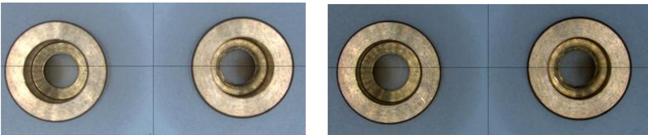
Fig. 8: A comparison of views of challenging shapes as seen through standard optics vs. telecentric optics. Sightlines to the bottoms of the deep holes are partially obstructed by the top edges of the holes when viewed off-center with standard optics (left). When viewed with telecentric optics (right), the entire surface of the bottom of the hole is visible.
