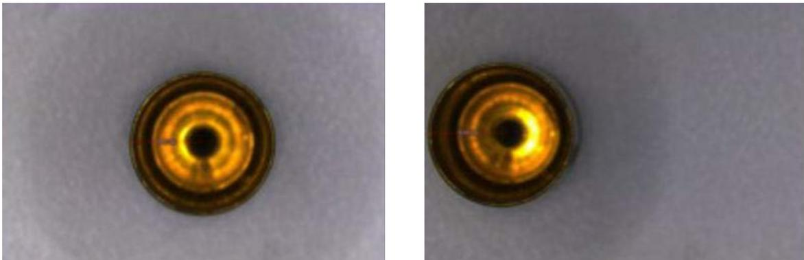
Fig. 3: Parallax error causing measurement inaccuracy. In left image, cartridge case is centered in field of view and on-screen measurement reads 4.62 mm from center of hole (far from objective) to edge of case (close to objective). In right image, same measurement is taken off-center and reading changes to 5.12 mm.
