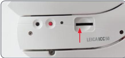
The camera's LED will turn green. The Leica ICC50 HD is now ready to capture images onto the SD memory card.
