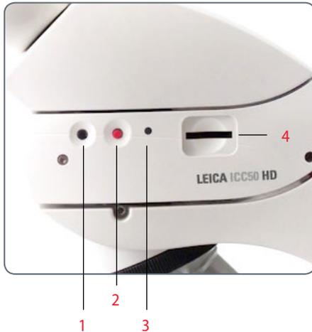
1. Black Multipurpose button: Press for 1 second – page through illumination settings. Press for 5 seconds – change mode between HD mode and PC Mode
