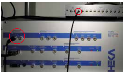
Figure 11: Trigger In: The scan start of the Leica TCS SP8 is triggered by an incoming trigger signal from a patch clamp amplifier (DA output signal). The analog output of the patch clamp amplifier is connected to the Trigger In 1 plug of the trigger unit.
