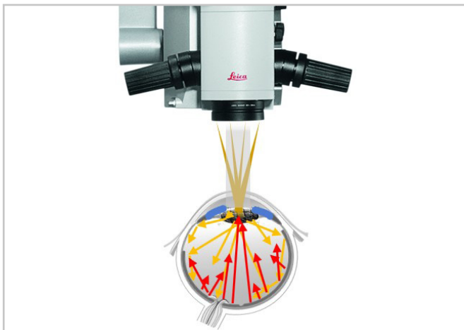
Fig. 4. Creation of a stable red reflex thanks to CoAx 4, coaxial LED illumination.
