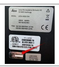
You can find the Leica identification label on the right bottom of the Mitaka stand. The Mitaka SN is behind the door on the left side.
