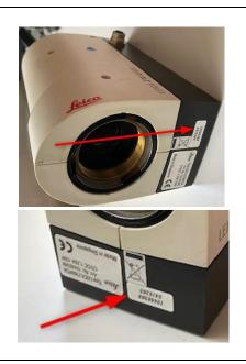
The label with the serial number is located next to the mount for the lens. It is helpful to remove the Optics carrier.
