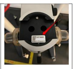
On the M320/M220 the identification label is on the top located. Therefore, you need to remove the tube first.
