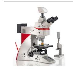
You can find the identification label on the back of the device.
